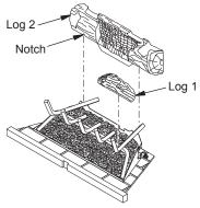
Figure 25 - Installing Logs 1 and 2
